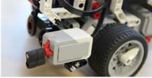
When the Touch Sensor is pressed, it closes an electrical circuit, allowing current to flow. If the Touch Sensor is released, the circuit is broken and no current flows.
